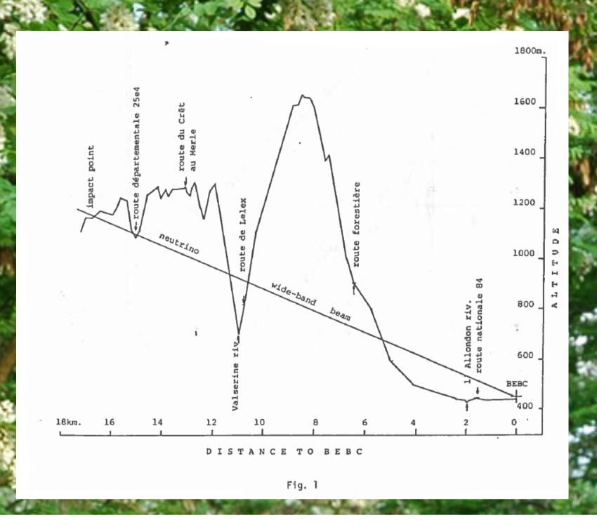
The first CERN SPS neutrino beam aimed at the JURA mountain, exiting at an altitude of 1200 m, 17 km from the production target
