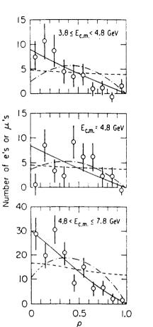
Figure 13. The scaled momentum spectrum of leptons from  $e\mu$  events in three energy regions. The solid curve represents the expectation of a 1.8 GeV/ $c^2$  lepton with V-A interactions. The dashed and dot-dashed curves represent the expectations from a 1.8 GeV/ $c^2$  boson with spin 0 and spin 1, helicity 0, respectively. (From the second paper, Ref. 13.)
