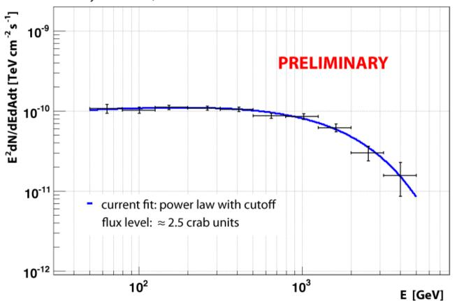
A VHE instrument (MAGIC) could measure the spectrum of a strong source at energies as low as ~ 50 GeV providing an overlap with a spaceborn γ instrument (FERMI)
