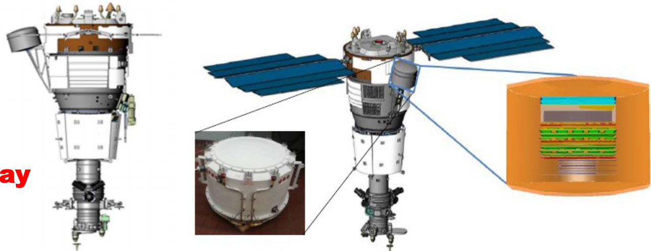
The NUCLEON detector on board of the satellite RESURS-P N2.
